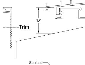
Apply a small bead of adhesive sealant to the underside of the vinyl sill (too much sealant may resist fully seating the sill angle).
