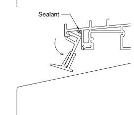
Apply sealant below adjustable foot and slide foot down to meet RO sill surface.
