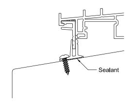
Alternate Non-Adjustable Application: If there is not enough room for use of the adjustable foot, or if prefered, trim sill angle in step 1 to match the opening dimenison "D". Apply sealant under vinyl sill and rotate sill angle into place without attaching adjustable foot. Seal bottom edge of sill angle and, if desired, use pan head screws to hold in place.
